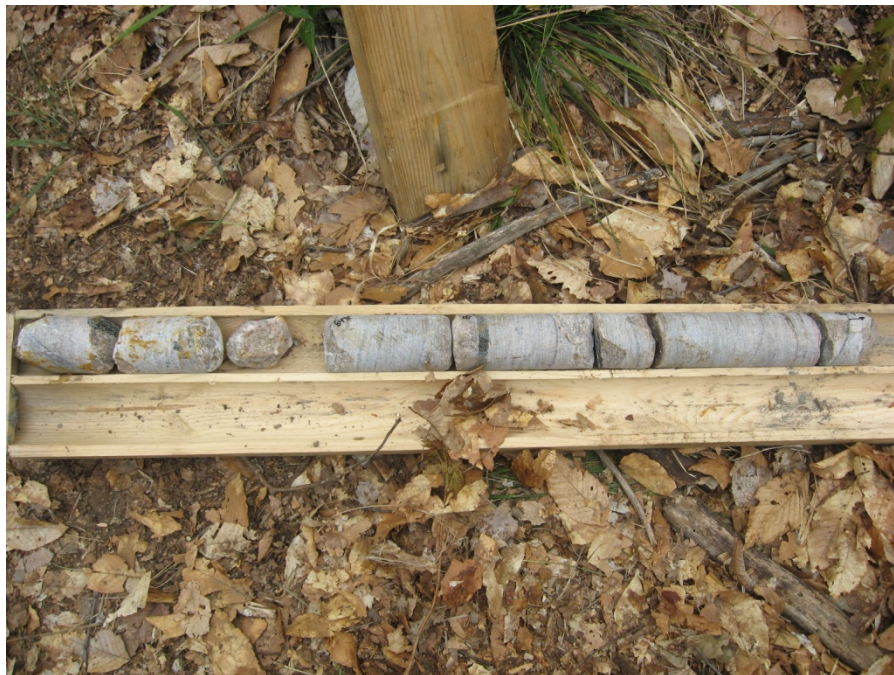
Photo 2 Monitoring Well MW5-06 Bedrock Core
